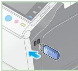
**1.** Plug in your USB in the ports located on the right hand side of the printer, near the touchscreen.
